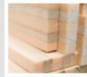
The paulownia wood core reduces the ski's weight by up to 30% for improved agility and handling while retaining control.
