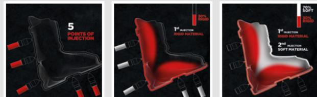
The entire HERO WORLD CUP and HERO range features the DUAL CORE technology. The process involves three injection points on the shell and two on the cuff. This technology can be used to accurately fine-tune the progressive flex, rear support and rebound. It also allows for highly effective lateral power transfer.
