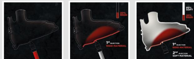
The DUAL CORE technology works in synergy with the Generative Design Grid. It makes it possible to reduce weight while retaining rigidity. This is essential to ensure a high level of skiability. On the ALLTRACK boots, the Dual Core technology is used on the lower part of the shell - which increases torsional rigidity and makes the boot easier to put on.
